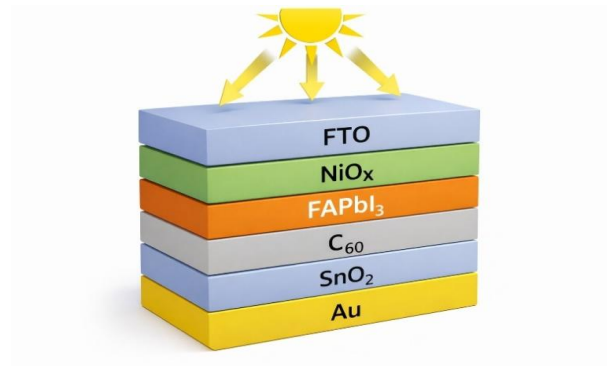
Figure 1. Schematic of FAPbI 3 based PSC structure used for simulation.
