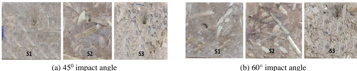
Figure 9. WF-WS samples non-PLA coated for air jet erosion test (a) 45° impact angle (b) 60° impact angle.
