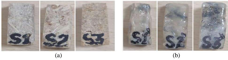
Figure 6. Samples of pin on disc test (a) Non-coated (b) Coated.
